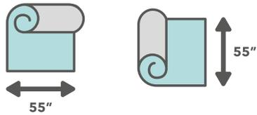
Fabrics **cannot be applied warp horizontal/railroaded** on panels with a **height greater than 48 inches** because panel height is greater than fabric width.
