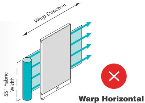
Fabrics **cannot be applied warp vertical** on panels with a **width greater than 48 inches** because panel width is greater than fabric width.
