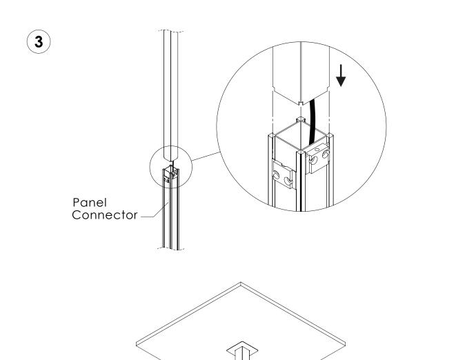
The Power pole is placed on top of the panel connector. Its weight exerts pressure and gives it the necessary support by securing it. No screws needed.
